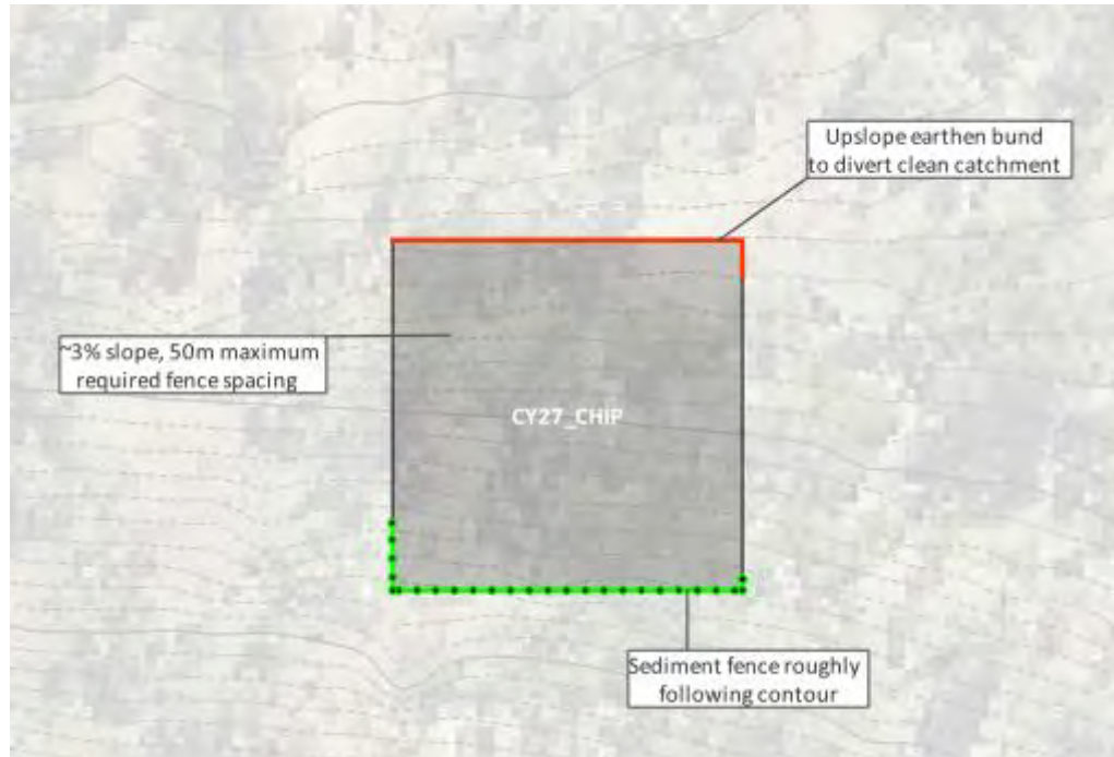
Figure 4.4 – Conceptual drill pad sediment management
