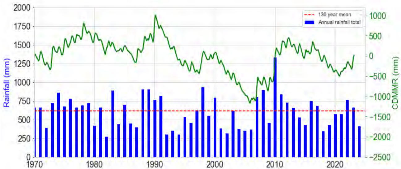
Figure 4.5 Total annual rainfall (blue bars), long-term annual rainfall mean (red dotted line) and CDMMR (green line) for the Project area
