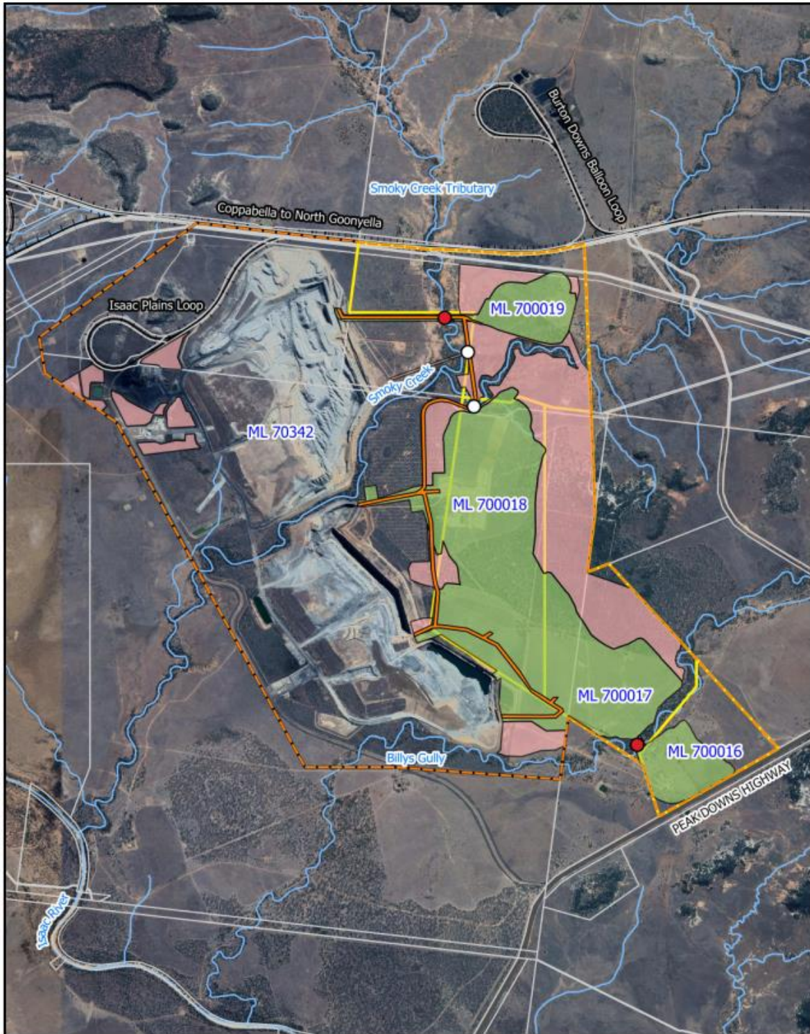
Figure 2: Project Layout and Disturbance Boundaries Legend ○ New Culvert Crossing — Watercourses □ Existing Isaac Plains Mine □ IPE Extension Project Area ● Upgraded Culvert Crossing — Highways □ IPE Mine Lease □ Haul Roads — Railway □ Isaac Plains Complex □ IPE Impact Area Scale @ A3: 1:40000 Date: 13/05/2020 Drawn: JAH/T DATA SOURCE: BACS CONSULTING GROUP 2020; OSPATHL 2020; The State of Queensland (Department of Natural Resources and Mines) 2020 BASE/
