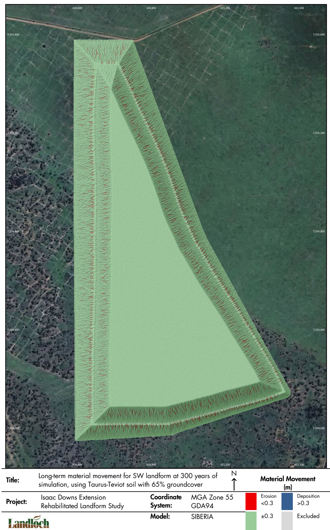
Figure D-4: Predicted material movement for the proposed Project rehabilitation landform when sheeted with topsoil (Taurus-Teviot) supporting 65% groundcover after 300 years of simulation – SW landform.
