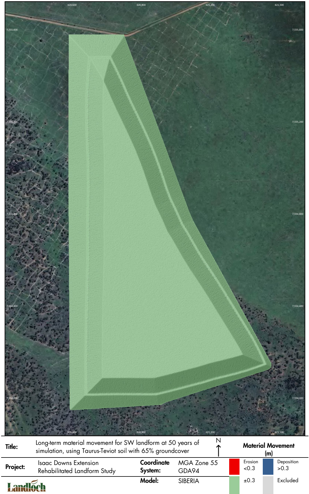
Figure D-1: Predicted material movement for the proposed Project rehabilitation landform when sheeted with topsoil (Taurus-Teviot) supporting 65% groundcover after 50 years of simulation – SW landform.
