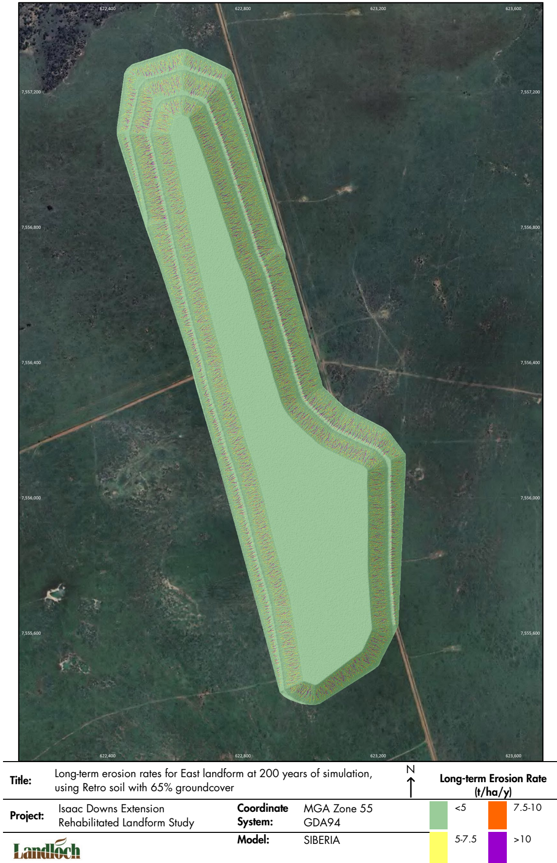
Figure D-23: Predicted average annual erosion for the proposed The Project rehabilitation landform when sheeted with topsoil (Retro) supporting 65% groundcover after 200 years of simulation – East landform.
