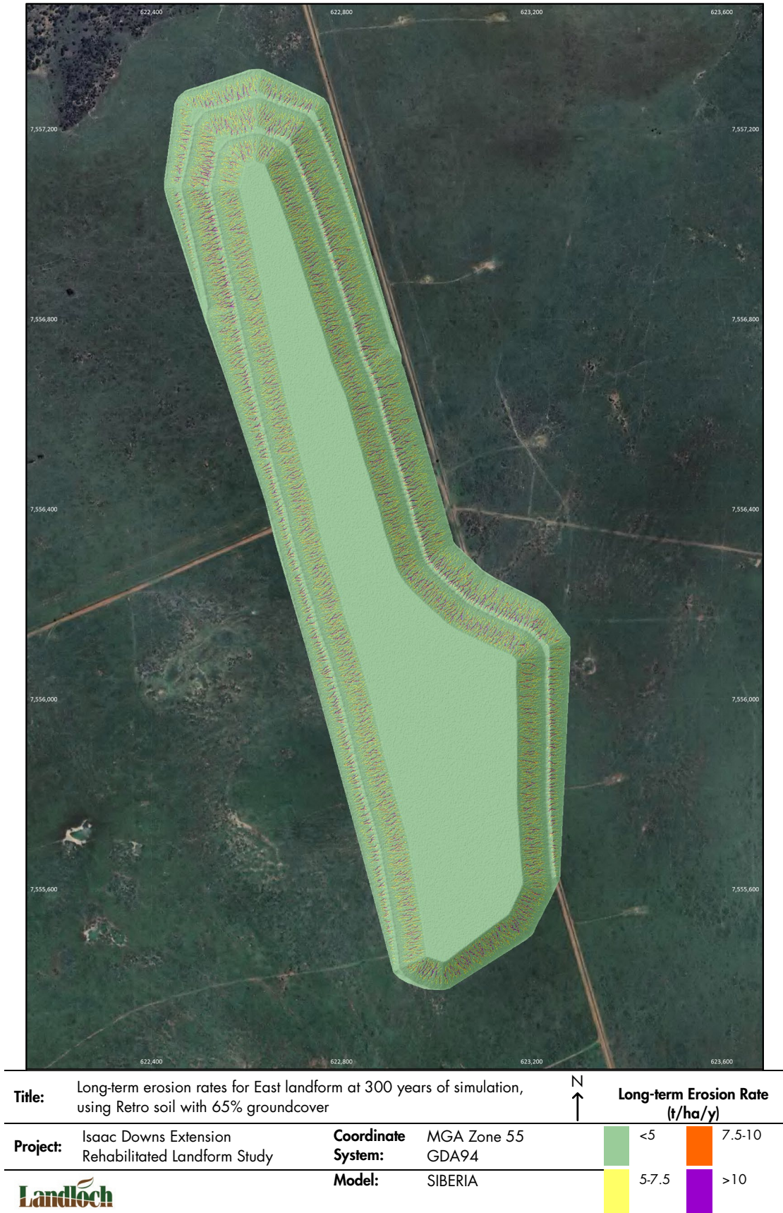
Figure D-24: Predicted average annual erosion for the proposed The Project rehabilitation landform when sheeted with topsoil (Retro) supporting 65% groundcover after 300 years of simulation – East landform.
