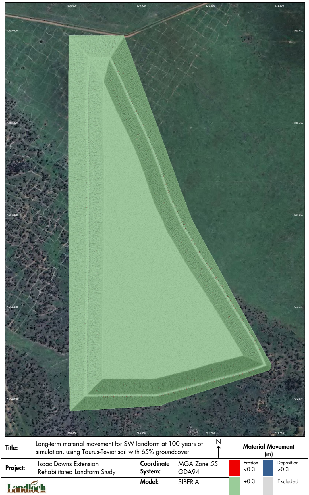
Figure D-2: Predicted material movement for the proposed Project rehabilitation landform when sheeted with topsoil (Taurus-Teviot) supporting 65% groundcover after 100 years of simulation – SW landform.
