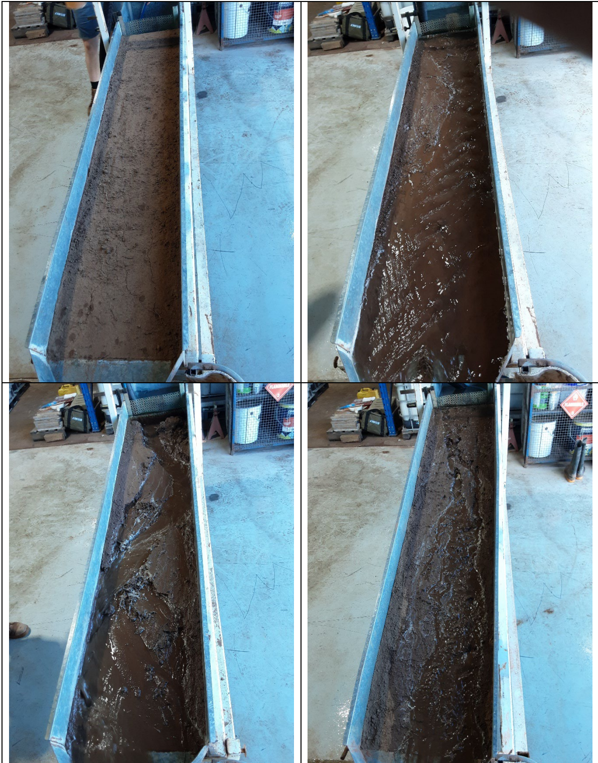
Figure A-9: Teviot overland flow studies before application of flow on 5% gradient flume (top left), and during application of flows on 5% gradient flume (top right), 10% gradient flume (bottom left), and 20% gradient flume (bottom right).
