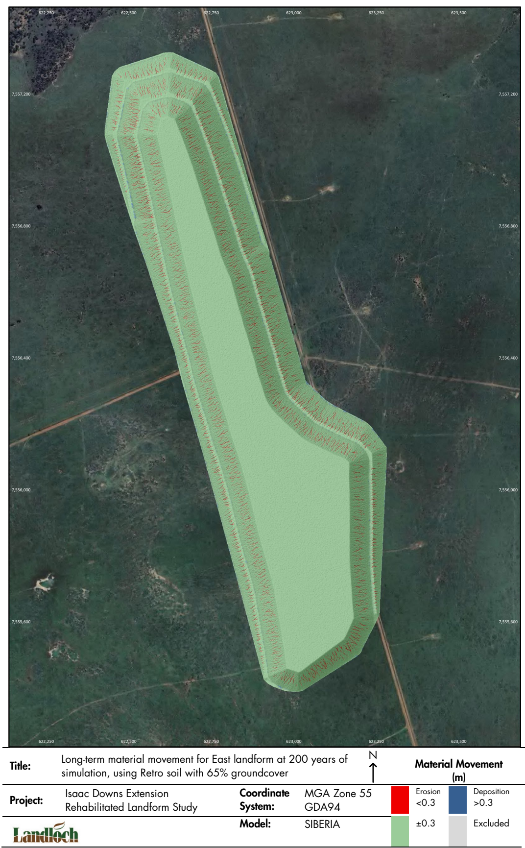
Figure D-11: Predicted material movement for the proposed Project rehabilitation landform when sheeted with topsoil (Retro) supporting 65% groundcover after 200 years of simulation – East landform.
