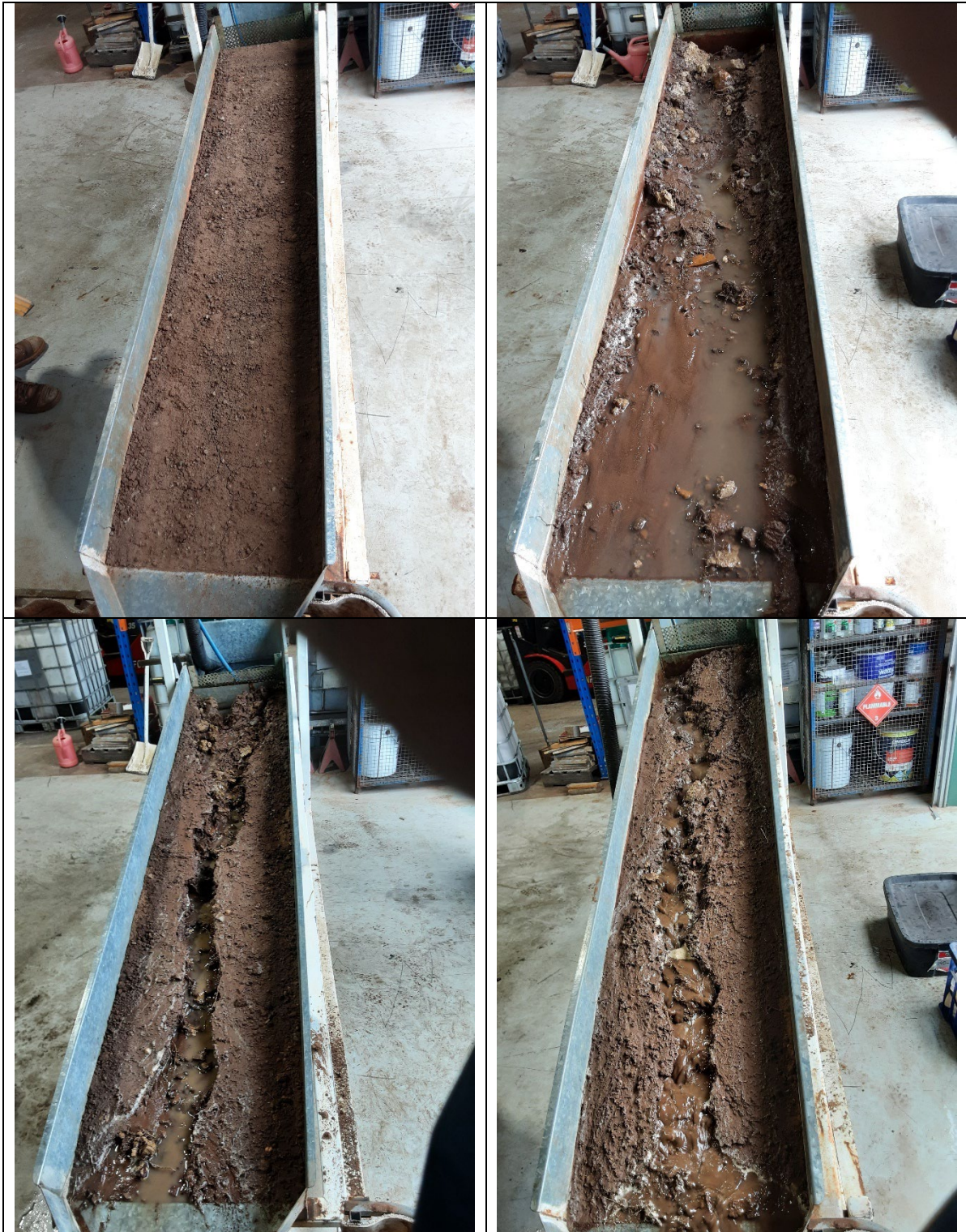
Figure A-7: Taurus-Teviot overland flow studies before application of flow on 10% gradient flume (top left), and during application of flows on 10% gradient flume (top right), 20% gradient flume (bottom left), and 30% gradient flume (bottom right).
