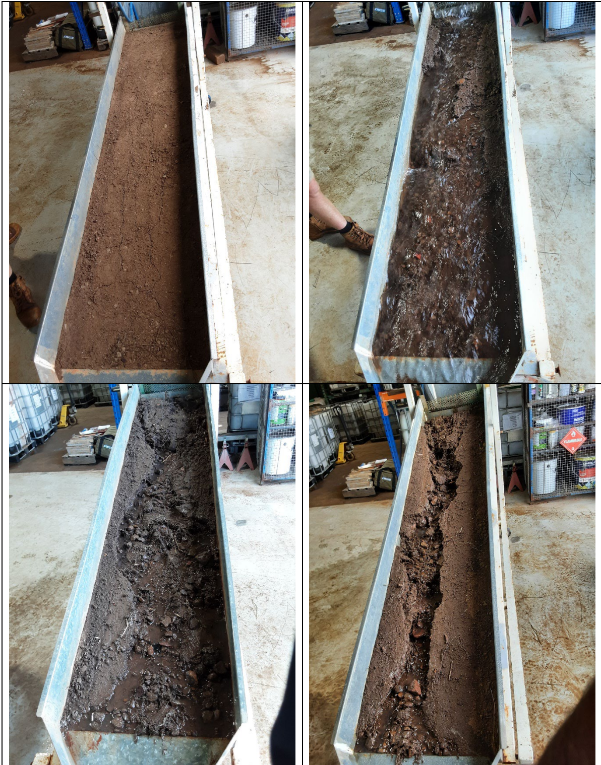
Figure A-10: Retro overland flow studies before application of flow on 10% gradient flume (top left), and during application of flows on 10% gradient flume (top right), 20% gradient flume (bottom left), and 30% gradient flume (bottom right).
