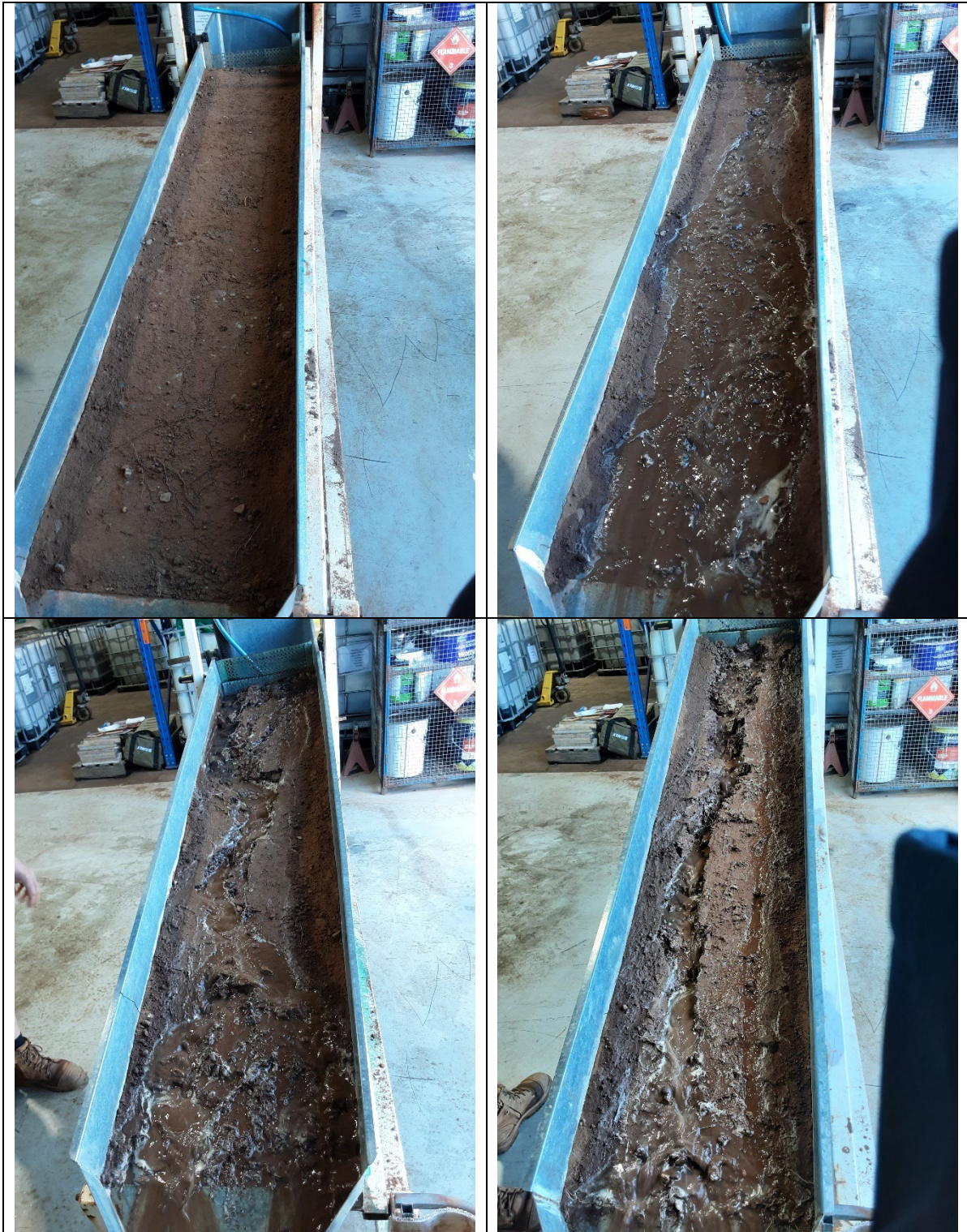
Figure A-6: Taurus overland flow studies before application of flow on 10% gradient flume (top left), and during application of flows on 10% gradient flume (top right), 20% gradient flume (bottom left), and 30% gradient flume (bottom right).
