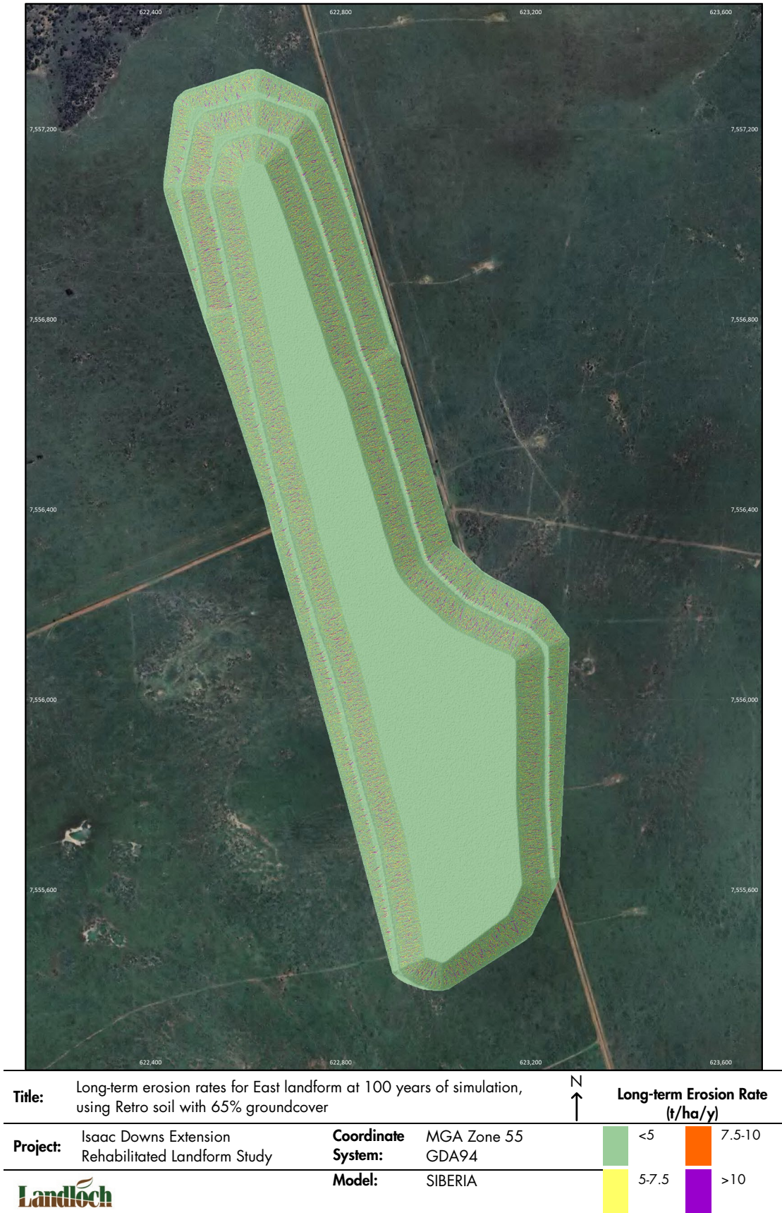
Figure D-22: Predicted average annual erosion for the proposed The Project rehabilitation landform when sheeted with topsoil (Retro) supporting 65% groundcover after 100 years of simulation – East landform.
