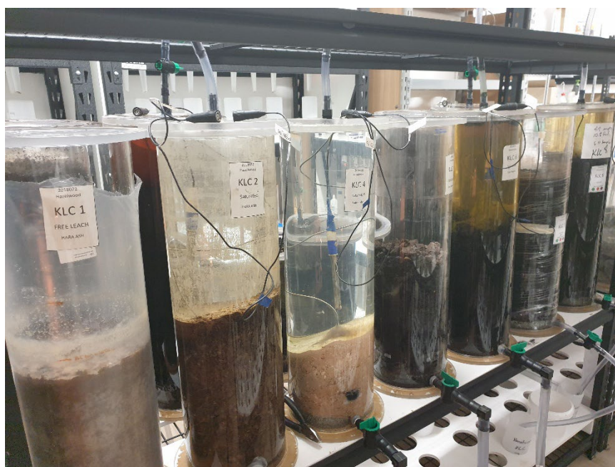
Figure 2-1: Kinetic leach column (KLC) tests for IDE at RGS Laboratory.
