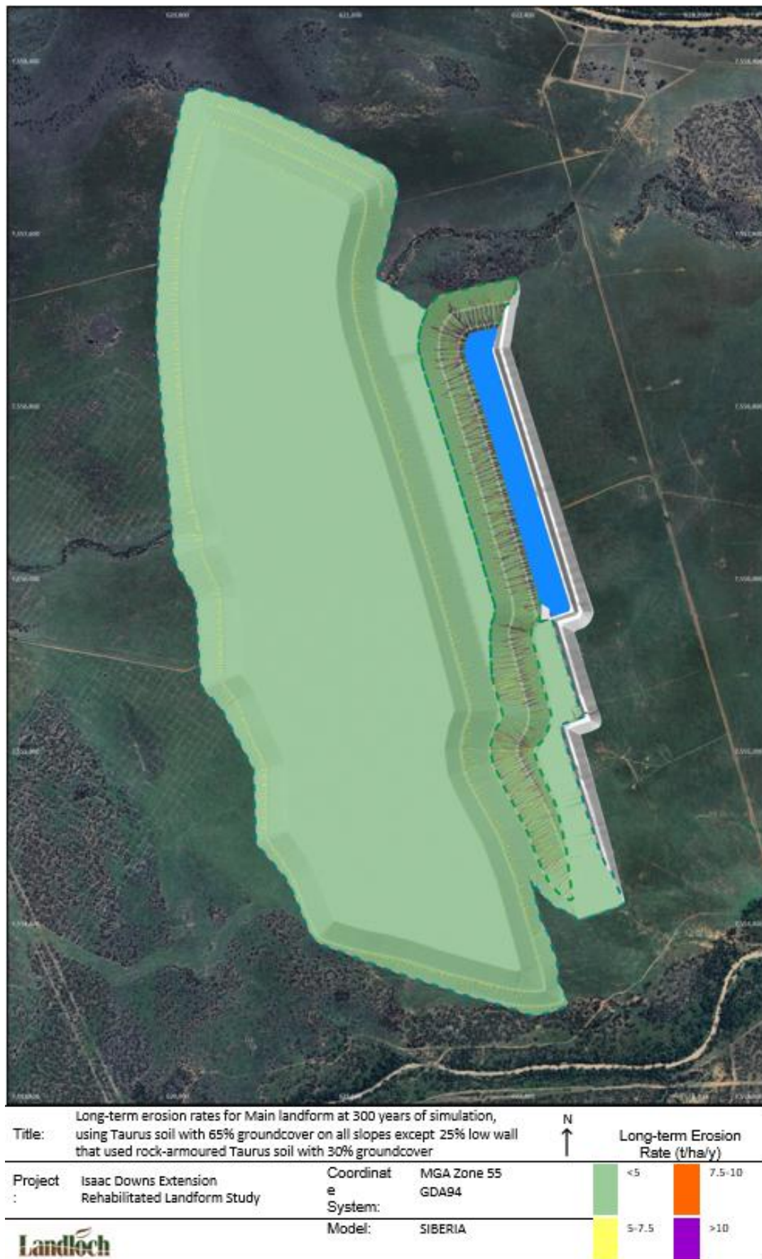
Figure 7-17 Long-term Erosion rates at 300 years for the Project's Main Landform
