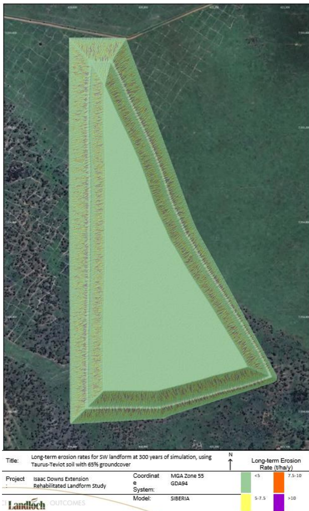
Figure 7-18 Long-term Erosion rates at 300 years for the Project's SW Landform
